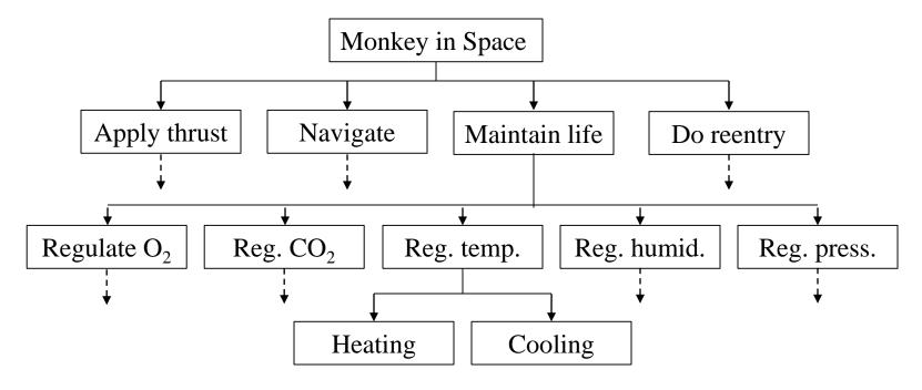
Systems can be thought of as a cascaded series of enabling functions
